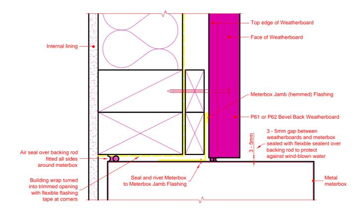
Note: Refer to the Bevel Back Cavity System Installation Manual for full details
