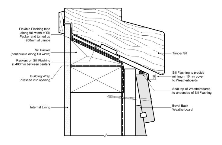
Important: Seal Sill Flashing to Flashing Tape (on Sill Packer) and also to Timber Sill with suitable cold sealant.
