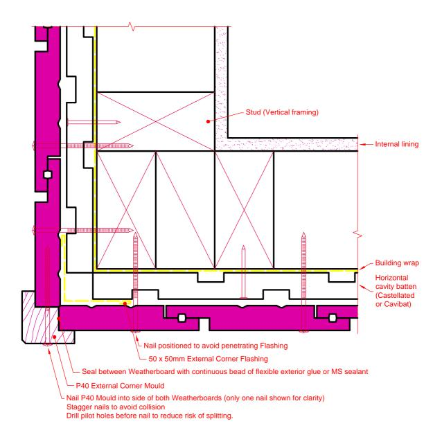
Note: Refer to the Vertical Shiplap Cavity System Installation Manual for full details
