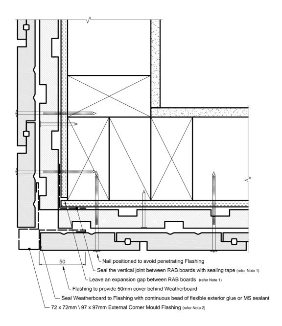
Note: Refer to the Vertical Shiplap Cavity System with Rigid Air Barrier Installation Manual for full details
