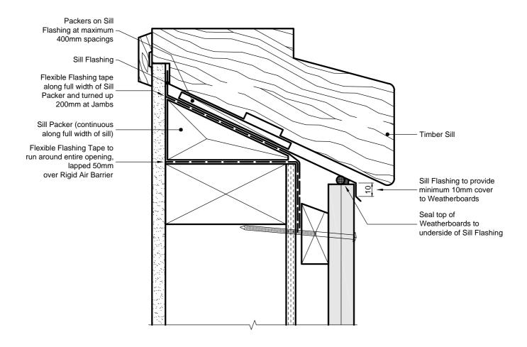
Note: Refer to the Vertical Shiplap Cavity System with Rigid Air Barrier Installation Manual for full details
